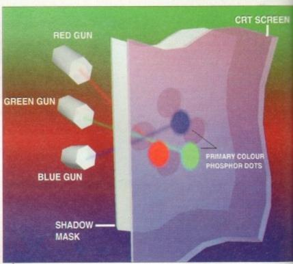
This illustration shows how the electron guns for each colour are aimed at their particular colou component of each phosphor triad. Note the Shadowmask screen to allow a degree of accuracy
